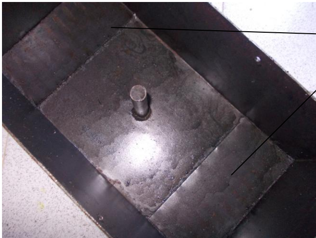
Fig4c. Detail showing two plates wedged in the basement of the mould. This small detail can not be seen in the basement of the concrete piece shown in fig 4 as it was required for better understanding of this functionality.
