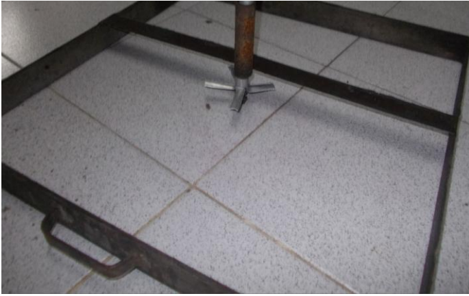
Fig5c. Mold of basement piece with guiding axis tube and inserted axis tube.
