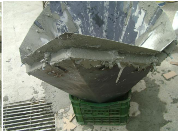
Fig3b. Mold filled. This was the first filling experience without using the bar for reinforcement shown in Fig 1h
