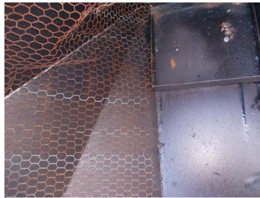
Fig2d. Mesh between the two funnel. It must not cover the mold of the rectangular hole
