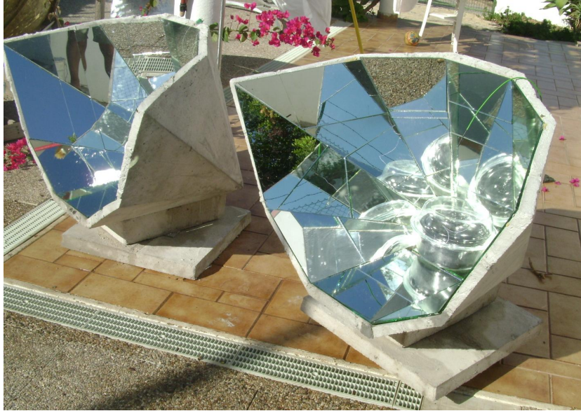
Fig. A – Two concrete funnel cookers, front view
