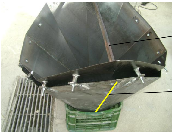
Fig1h. Interior and exterior funnels joined and ready to be filled with concrete mass
