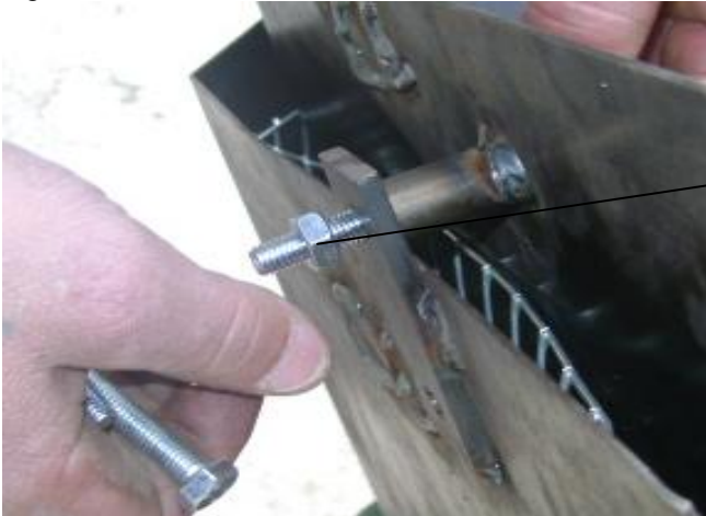
Fig1g. Detail of joining interior with exterior funnels
