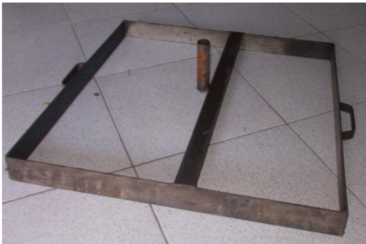
Fig5a. Mold of basement piece with guiding axis tube shown in fig 5b. Walls of the mold are bars with 50 mm, thickness 4 mm. the square bottom is 550mmx550 mm and the square top is 555 mm. The guiding tube is center and it is welded to the bar in the middle with thickness 4 mm, with 35 mm and length 550 mm. Nominal size of the guiding tube is 1/2" (15 mm), outside diameter 21.3 mm and inside diameter (standard size) 15.8 mm and height is 100 mm.
