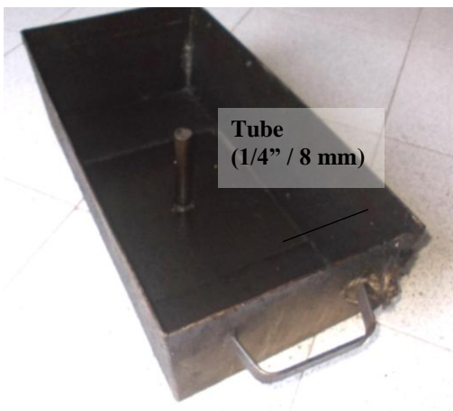
Fig4a. Box with tilted walls (vertical slope 7.5mm/115 mm. Bottom 460mmx225mm, top 475mmx240mm, height 145 mm. Height of the tube 110 mm. The nominal size of the tube is \frac{1}{4} " (8 mm), outside diameter is 13.7 mm and inside diameter (standard size) is 9.2 mm. The tube is centered. Bottom and walls of the box are made in steel sheet with 2 mm thickness or between 2 and 3 mm.
